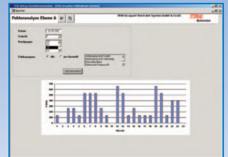
Level 6 displays the fault rate per shift in a 15-minute-cycle. It may be possible to identify faults relating to time here (e.g. at the beginning of shifts, after breaks, etc.).
